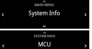
"System Info" displays information about current MCU, LCD and FPGA firmware versions.
